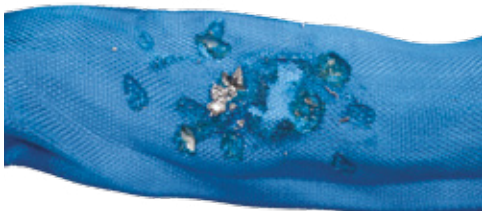
ROUNDSLING WELD SPLATTER
