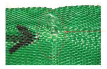
THE DAMAGE: **Holes/Snags/Pulls** exposing internal core yarns.
