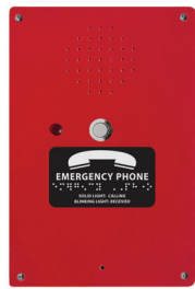
Model Number: 2100-984LR Size: 9-7/8" H x 6-5/8" W x 3-1/4" D Style: Red, NEMA 4, Fiberglass, Exterior Rated Options: Strobe Interface & Relay, Mushroom Push Button
