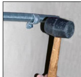
11. Insert the Spear-Tipped Support Arms into the Front Bar and attach to the Camel Back Hinges with the hardware provided.
