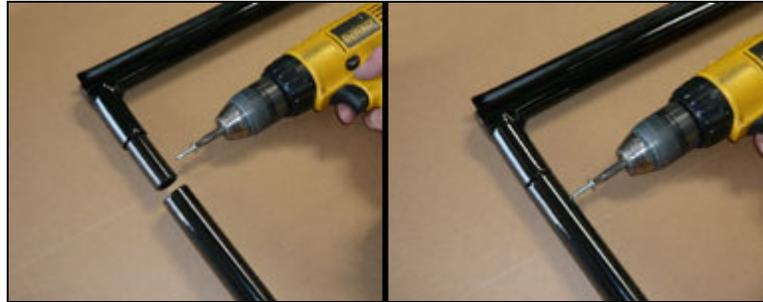
5. Assemble the Center Rafters and Front Bar. Attach the Front Bar and Outer Rafters together by driving the self-tapping Tek Screws into the pilot holes.
