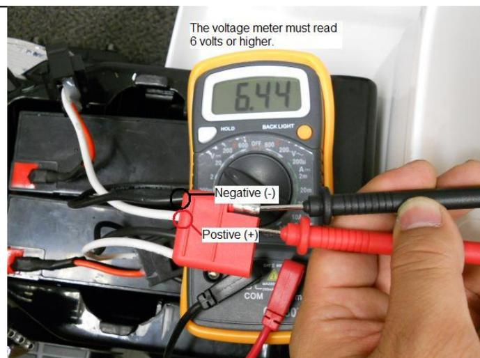
powering the Police Patrol 12V. Each battery will need to be tested individually for proper assessment. The reading off each battery should read 6-volts or higher.
