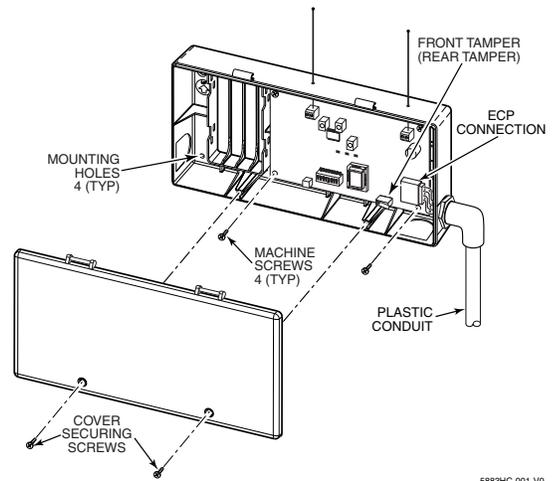
**Figure 3: 5881ENHC UL Commercial Fire Installation**
