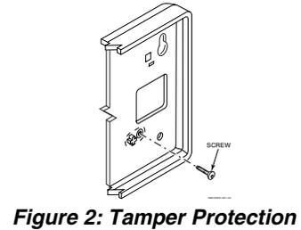
**Figure 2: Tamper Protection**
