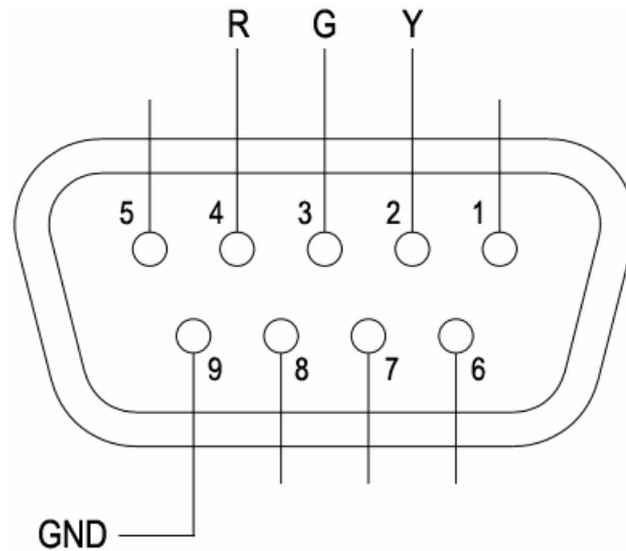
The RED light is on when connecting the terminal “R” with “GND”, and goes out when disconnecting.
