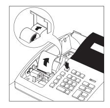
3. Depress the "**FEED**" key until the paper begins to advance through the printer.
