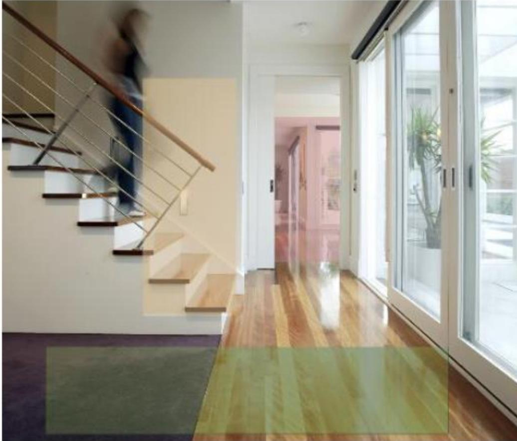
The configuration seen above minimizes effects from the always-changing natural light coming in through the sliding glass doors on the right. It focuses on three areas that the user needs monitored: the stairwell, the hall area at the foot of the steps and the hallway beyond the doors.
