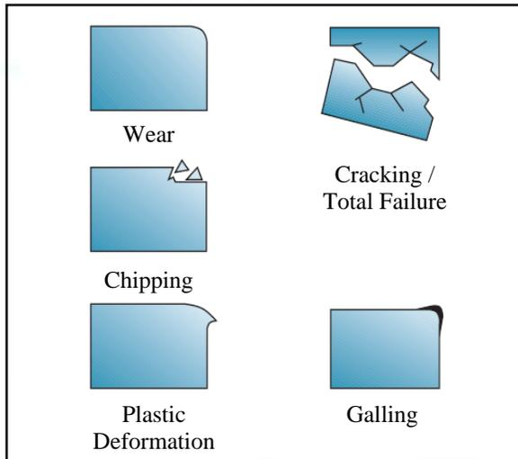
Figure 2. Common failure mechanisms of cold work tools
