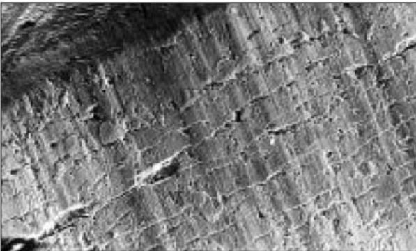
Figure 4. Photograph of D2 worn by adhesive wear.
