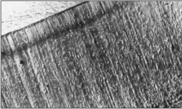
Figure 3. Photograph of D2 worn by abrasive wear.
