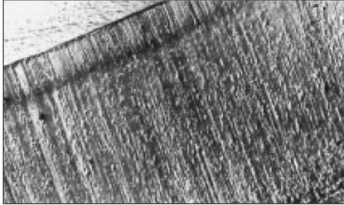
Figure 3. Photograph of tool worn by abrasive wear.
