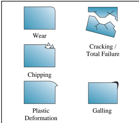
Figure 2. Common failure mechanisms of saw blades
