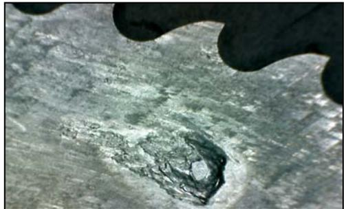
Figure 5. Photograph of tool worn by galling.
