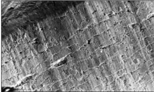
Figure 4. Photograph of tool worn by adhesive wear.
