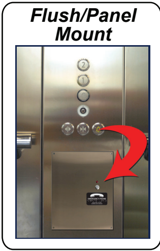
Model Number: 2400-808SS Plate Size: 12-1/2" H x 9-3/4" W x 2" D Back Box: 8" H x 6" W x 3" D Style: Brushed Stainless Steel Option: Mirrored Stainless Steel
