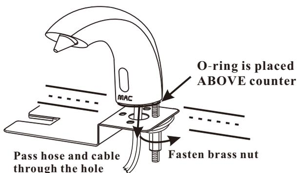
Before installing the stainless steel bracket please make sure that there will be plenty of space for the pump housing. Please exercise special care not to cut the Soap hose or damage sensor cable while fastening the brass nut.
