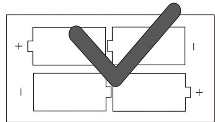
Place batteries in battery box according to drawings above.
