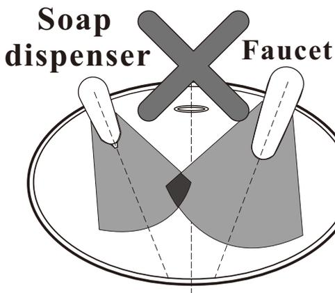
Keep sensor range adjustment within 4 inches away from center of spout. This can only be done with optional remote control.
