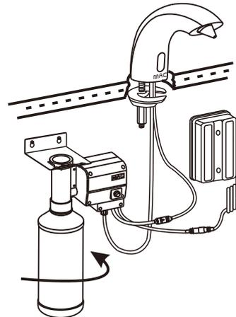
3. Affix the bottle with full soap onto the pump, and do not over tighten..
