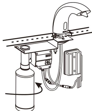
3. Affix the bottle with full soap onto the pump, and do not over tighten..
