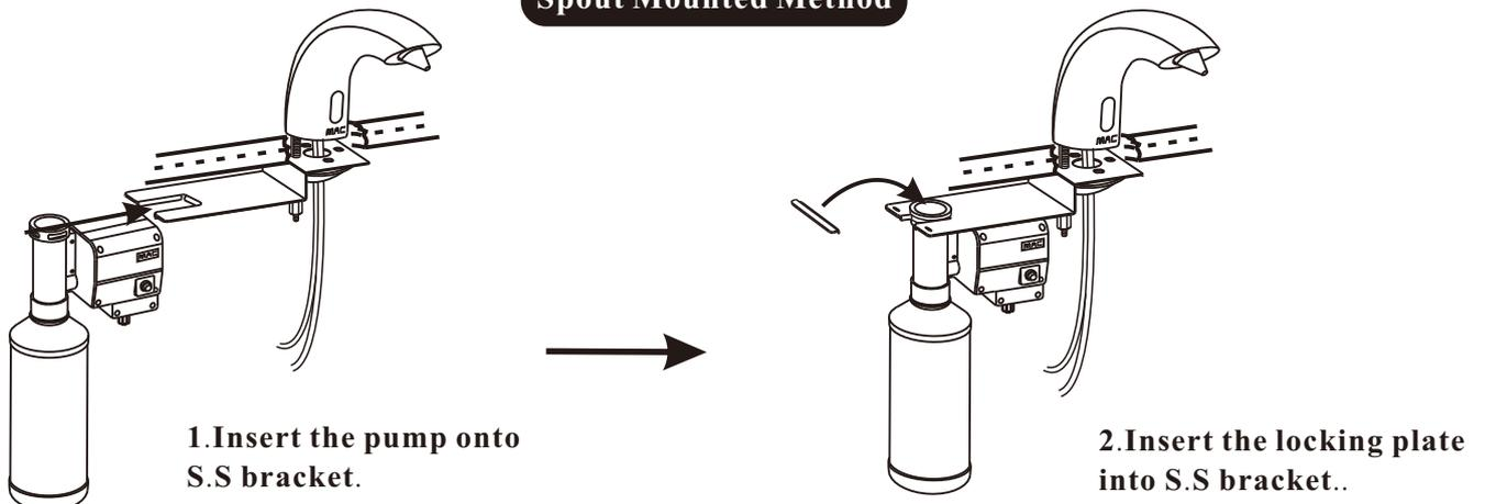
1. Insert the pump onto S.S. bracket.
