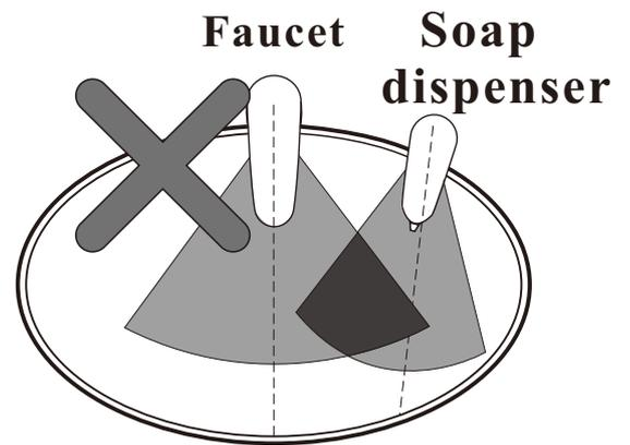
Installing electronic soap dispenser and faucet with intersecting centerline might lead to accidental activation of either or both.
