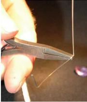
Now place the mark on your chain nose pliers at the base of the 90-degree bend and bend the wire again 90 degrees.
