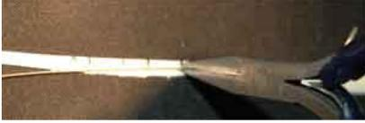
Pick up the wire with the pliers and bend it upward 90 degrees.
