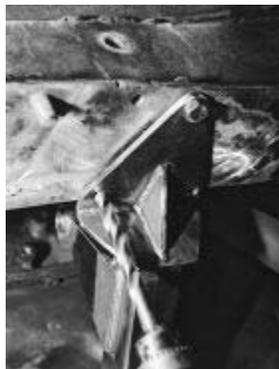
Additional mounting holes are then drilled after the crossmember is mocked in place.
