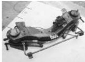
The Walton six-cylinder crossmember is designed for use on stock frames with Mustang II-style suspensions, although Walton says it may work with stock suspensions if a later-model steering box is employed.
