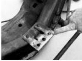
Radiators on '41-48 Chevys are supported by a bracket on the front suspension crossmember. With the stock crossmember gone, Todd designed this bolt-in support.
