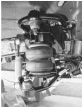
As noted in the text, this particular car was fitted with an airspring IFS setup from TCI. We were unable to document the installation, but here's what the finished product looks like. Walton tells us that Mustang II-style suspensions fit Chevys of this era particularly well, and are relatively simple to install.
