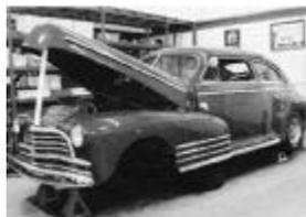
It's no surprise to see a six-cylinder in a '46 Chevy, but the inliner residing under this hood isn't a splash-oiler 216, but a more modern 250. Walton Fabrication is now offering the parts to make this a relatively simple swap.
