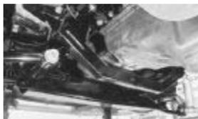
Here's a look at how the engine crossmember fits with the TCI suspension installed. This is looking from the rear toward the front.
