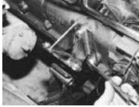
Adapter brackets allow the use of V-8 engine mounts on the six.
