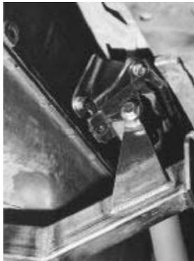
Here's a look at the crossmember, engine mount, and adapter bracket on the driver side, as viewed from under the [car](#).
