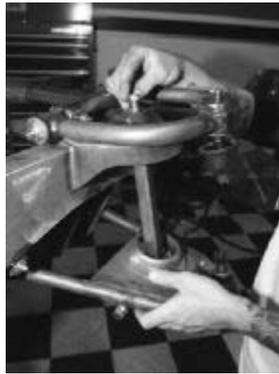
Trying to install coil springs on an empty chassis without them flying out across the shop can be very difficult, so some dummy struts were cut, drilled, and installed as a temporary solution until we got some weight on the chassis.
