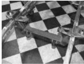
The engine mounts were welded in next. Walton has specifications for most popular and even some exotic engine choices when it comes time to set-up the mounts. If you want something they don't have specs for, they'll work with you to get it right. This setup is for a small-block Ford.
