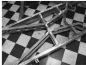
We were extremely impressed with the X-member. It's large and no doubt adds a ton of rigidity to the chassis, but it still provides plenty of clearance for the driveshaft and exhaust.
