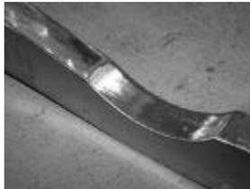
The result was an amazingly smooth appearance from the front of the rail to the rear. Here you can see the mild C-notch incorporated into the rear rails.
