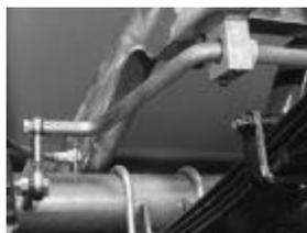
An optional 3/4-inch rear antisway bar can be ordered to go along with the front bar and will do a lot to making the truck more enjoyable to drive through a twisty canyon. The bar attaches to the provided mounting points on both the frame and via heims to the axle housing.
