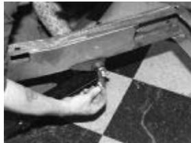
Jason slid the rearend under the chassis, fished the leaves under the housing, and bolted them to the hanger and shackle. Walton offers a variety of rear suspension choices, including a four-link with either coilovers, 'bags, or ShockWaves. If you want to supply a Corvette or Jag IRS, those can be incorporated too.
