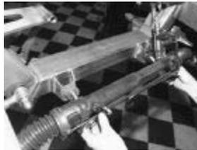
The power rack was installed onto the mounting points on the front of the crossmember, and the tie-rod ends were bolted to the spindles.
