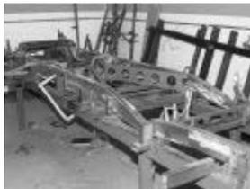
The finished framersails were then attached to the frame jig, and the crossmembers were clamped in. The center X-member really ties it all together into one strong piece.
