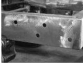
Here you can see the two sets of mounting holes that can be used for the rear bumper. Each set of holes uses the stock brackets, but the upper set mounts the bumper up higher and closer to the body.
