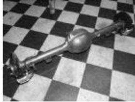
The 9+ rearend from Currie was built specifically for this chassis. It is 100-percent brand new and features the upgrade to Explorer disc brakes. Since we will be running an overdrive trans, we equipped the rearend with a 3.70:1 third member with 28-spline axles.
