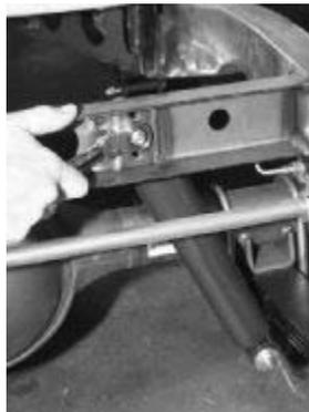
The shock bolts to the crossmember and has plenty of clearance all around to accommodate a variety of different shocks, such as some of the adjustable ones on the market.
