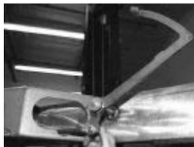
The brake pedal was bolted up to the pivot point and connected to the pushrod.
