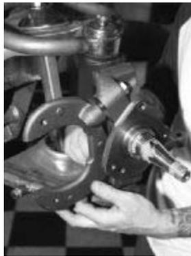
The spindle assemblies come pre-assembled with the rotor and caliper in place. The spindles feature a 2-inch drop, but if you so desire, standard ones are available. We disassembled the assemblies so you could better see the components used.
