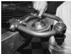
Our Tech Center master mechanic, Installation Jason, began the assembly by installing the upper tubular control arms. Once again we opted for the standard pieces, but stainless ones are available if you'd like to step up.
