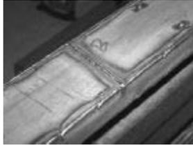
The inside wall that completes the "box" was put on in a few pieces. The sections with welded nuts for running boards or other accessories were welded in first. Then the open sections were filled in with plate steel.
