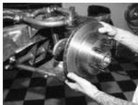
The front brake system we are using features GM '78-up mid-size passenger car calipers with 11-inch rotors. Larger 12- and 13-inch Wilwood brakes are an option. Either system can be matched to the Ford 4.5-inch bolt pattern or the GM 4.75-inch.
