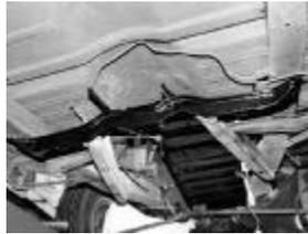
Moving under the car, here's a look at the original transmission crossmember. As you can see, it attaches to the frameraills as well as two braces that angle back from the front of the frame.
