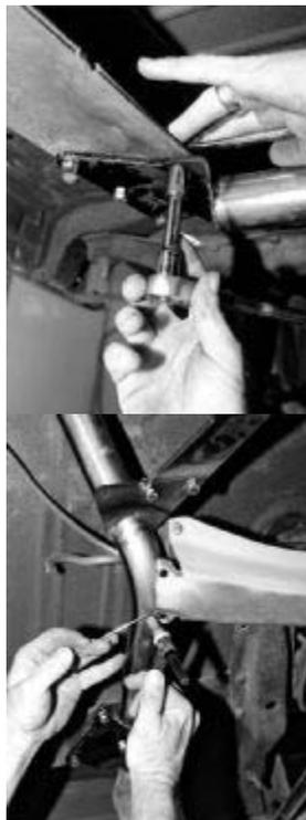
The crossmember bolts to the top side of the two center braces and is welded to the ears on the bottom of each brace. The ears may have to be bent slightly to fit snugly against the crossmember.
