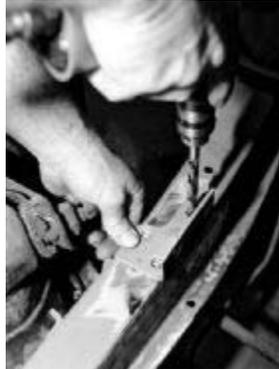
The factory engine mount brackets are riveted to the frame, and should be removed prior to installation.
