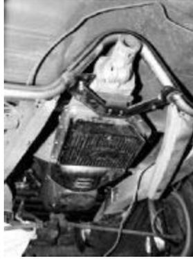
The transmission fits just as well. The drop-out mount allows for easy tranny removal and can be oriented in several configurations to accept a variety of transmissions.
