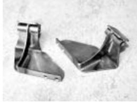
The engine mounts are simple, sturdy and well constructed. They'll work for both small-block and big-block Chevy engines (although big-blocks may require relocation of the radiator). The holes in the lower flange help align the mounts on the frame.
