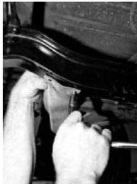
The Walton Fabrication crew has found from experience that some '49-54 Chevy transmission crossmembers were riveted in place, while others were bolted. Regardless, all the fasteners will have to come out before the old piece is removed. Even then it might take some coaxing with a hammer.
