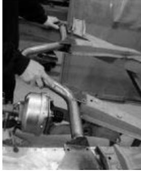
Todd Walton sets the new crossmember in place, illustrating how the diagonal frame braces meet the new piece. Test-fitting will reveal whether further trimming of the braces is necessary.
