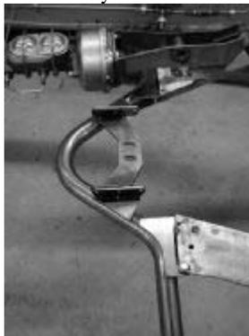
Here, the frame has been turned over so that it is right-side up and the crossmember is fully installed. The trans mounting bracket is removable, which allows it to accept a number of popular transmissions. The position shown is for a 700-R4, but by using other mounting holes and/or reversing the position of the mounting bracket, the crossmember can also be used with TH350, TH400, 200-4R, and Powerglide as well as most popular GM manual transmissions.
