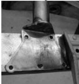
Once the frame braces clear the new crossmember, it is lined up with the factory holes in the framersails. All five of the holes should already exist, though one hole is slotted to accommodate factory variation so that no additional drilling or cutting should be necessary.
