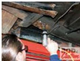
Walton Fabrication's instructions let you know exactly what size to drill out the rivet holes to, in order to accept the new hardware.
