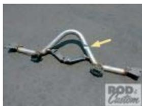
With the motor mounts completed, the transmission mount was next. Walton Fabrication offers this crossmember that replaces the original, the central saddle is adjustable for a wide range of GM transmissions. This particular car was to be fitted with a 200-4R overdrive trans, which owing to the shape of its sump pan required a different saddle, as well as a notch in the crossmember (arrowed) to allow
