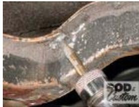
Removing the rivets that secure the stock crossmember is a dull and tedious job if you drill and punch them out by hand. The rivet heads were removed with an air chisel before a punch was used in the air hammer to drive out the rivets, making for a quick, if noisy job. With all the rivets removed, the crossmember was tapped rearward and removed.
