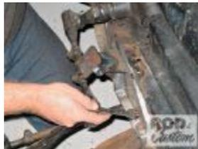
With everything cleared for the V-8 to fit, engine mounts were in order. Walton Fabrication manufactures these neat mounts that are simple to locate without requiring a dummy motor (or your intended one for that matter) and even come with instructions. The Walton mounts bolt in place using a pair of the front suspension mounting bolts for location. Before they were welded, they were clamped to the frame to close up any small gaps.
