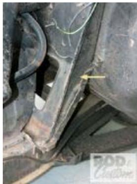
With the stock straight-six motor removed, these two ribs (passenger side arrowed) running from the top of the firewall to the chassis mount below have to be removed in order to fit a small-block Chevy.
