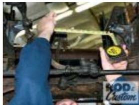
The distance between the mounts was double-checked as recommended in Walton Fabrication's instructions.
