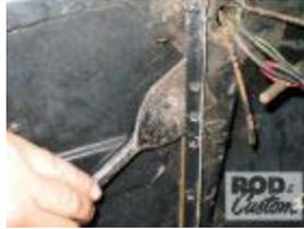
The majority of the rib was cut away using a cutoff wheel, leaving the lip attached to the firewall. Using a spot weld drill, which removes the weld but doesn't penetrate the layer of metal below it except for a small dimple, the spot welds were drilled out then the lip was pried from the firewall using a chisel.
