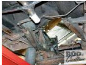
You should end up with the stock crossmember complete with the emergency brake actuating arm on the garage floor, and the underside of your car should look like this with it removed. Time to clean up around all the mounting holes.
