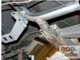
Walton Fabrication recommends you bend up the ears on the stock chassis outrigger sections and weld them to the new crossmember, though this was left until the end of the installation in this case.
