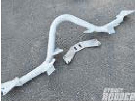
*The Walton tubular crossmember is designed to bolt in and incorporates a versatile mount that accepts six transmissions, including aluminum Powerglides, TH350 or TH400, the 700-R4, 4L60E, and a T-5 manual trans.*
