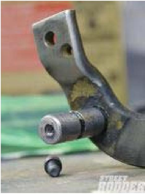
*The most difficult part of the master cylinder install was drilling and tapping the pivot shaft. This is important as this bolt retains the assembly securely in the new bracket.*
