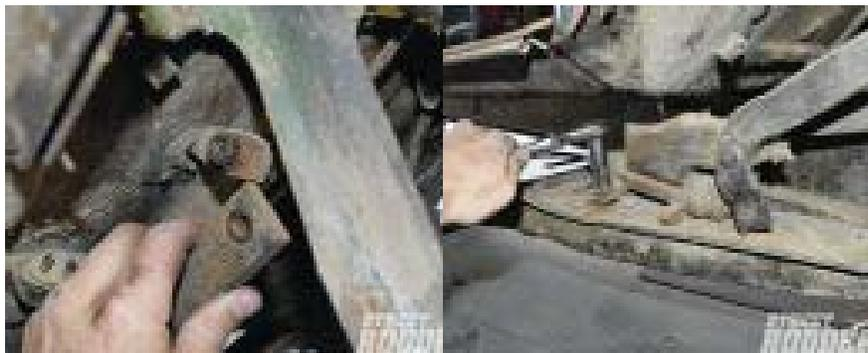
*Once again, it was out with the old and in with the new. We removed the intermediate pedal bracket from the pedal itself and then removed the original master cylinder assembly.*
