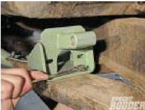
*The bracket simply mounts to the chassis in the same location as the original equipment. Once the bracket was retained, the master cylinder was installed.*
