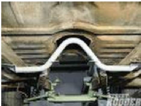
*With the crossmember in place, you can see that its design and construction will not only make installing our new small-block and trans easier, but it will also add strength to the frame.*
