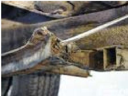
*Once we cut the factory crossmember away from the support brackets, you could see why even southwest cars rust. The frame supports were packed solid with dirt.*
