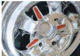
Real knock-off Halibrand wheels roll on custom-machined spindles and each hoop is wrapped in Mickey Thompson tires.
