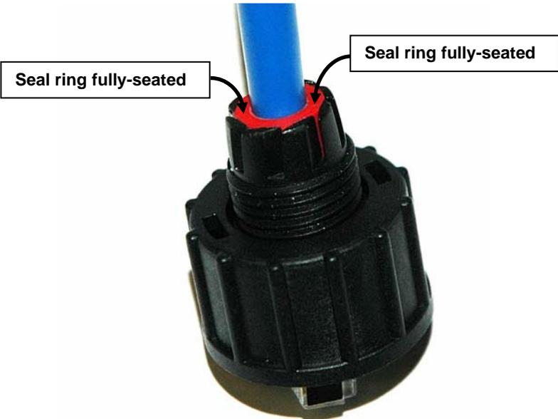
6. Plug the assembly into the socket on the E-STS-O and secure the screw nut. Then apply the sealing nut and securely tighten.
