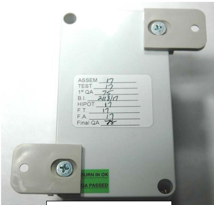
Brackets and screws installed.
