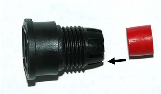
2. Strip the CATx shielded cable jacket (6mm-7mm O.D.) approximately 1/2" and insert the cable through the sealing nut, screw nut, and housing. (Note: Heat shrink tubing can be applied to cable to increase the O.D. of the CATx cable to 6mm-7mm.)
