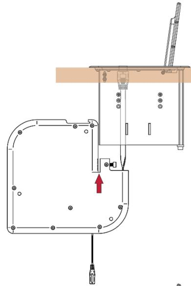
2. Use the appropriate Allen key to fix the **KRT-3** by tightening the Allen bolt firmly in place and pass the retracting cable end through the cable pass-through bushing.
