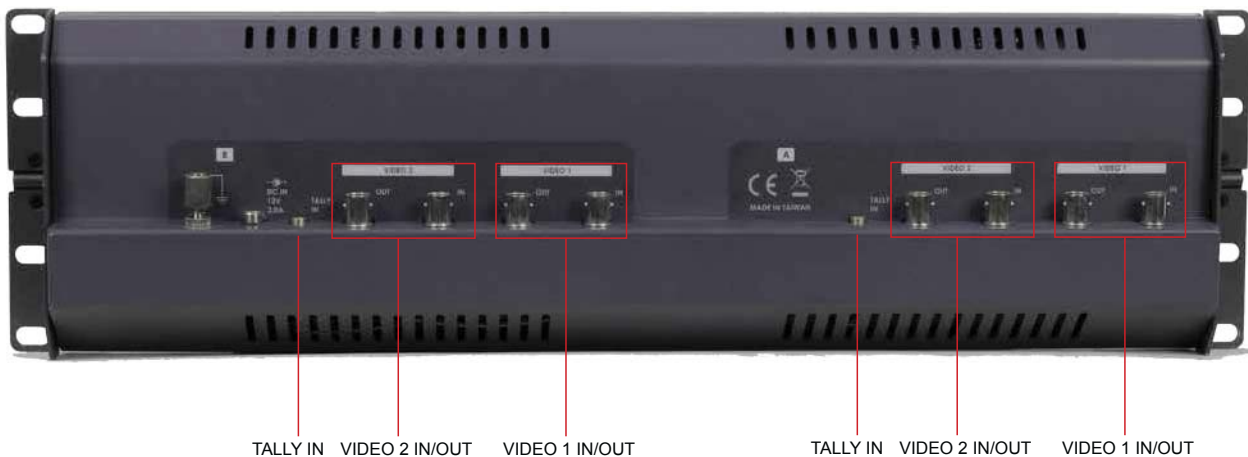
TALLY IN VIDEO 2 IN/OUT VIDEO 1 IN/OUT TALLY IN VIDEO 2 IN/OUT VIDEO 1 IN/OUT
