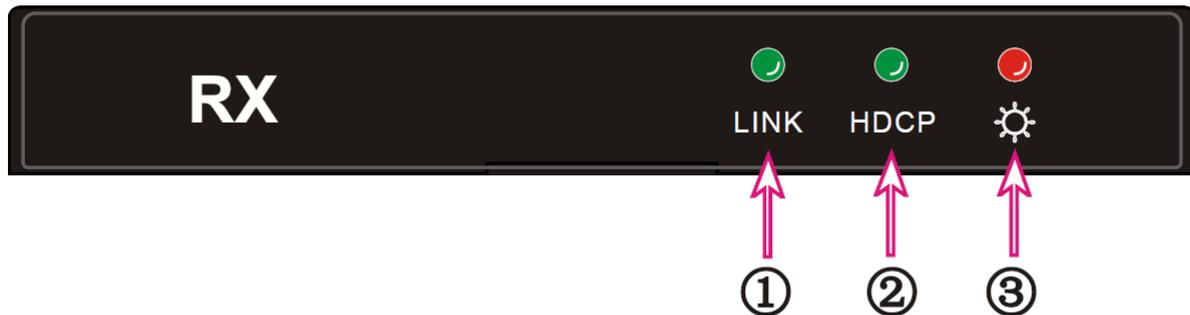
1. **LINK LED:** The LED illuminates green when there is a successful link between the transmitter and the receiver. It blinks green when there is a problem with the link and is off when there is no link.
