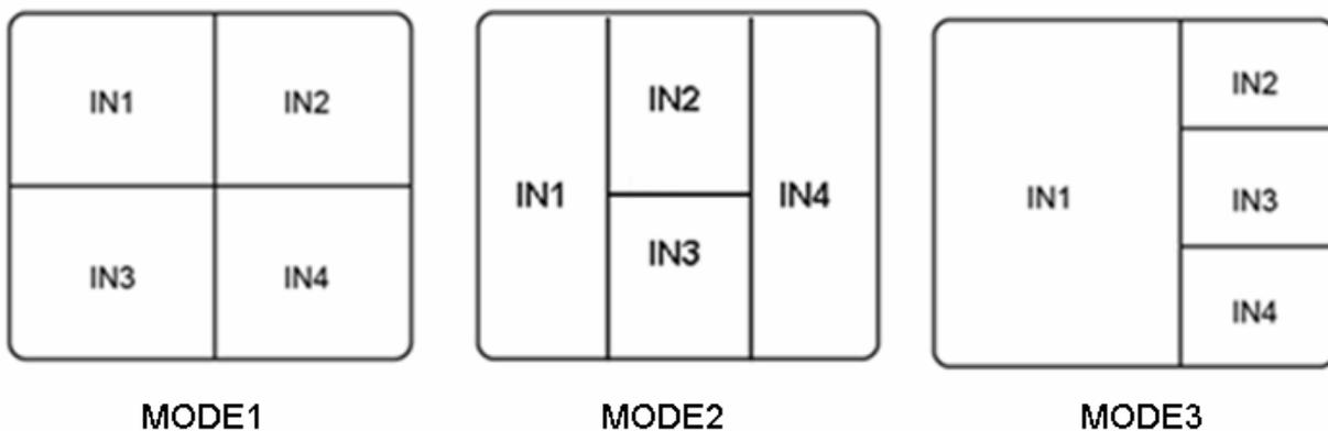
MODE3: It can choose the any of the HDMI input as the Main Picture( audio and video simultaneously) by press the matched mode button.
