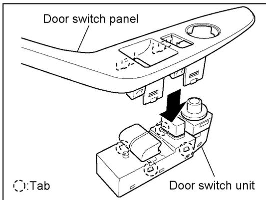
2. Assemble the door switch unit to the new door switch panel by engaging the tabs (4 places).
