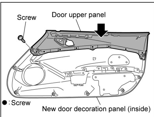
4. Install the door upper panel which was removed in step 3 to the new door decoration panel.
