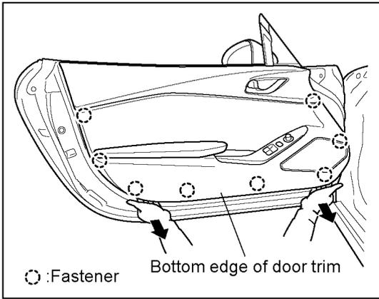
6. Insert your fingertips into the left and right parts of the bottom edge of the door trim as shown in the illustration at left to disengage the fasteners (8 places).
