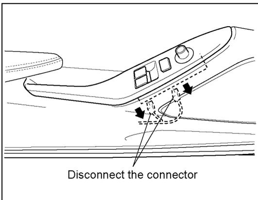
9. Disconnect the door switch connector, and then remove the door trim from the vehicle door.
