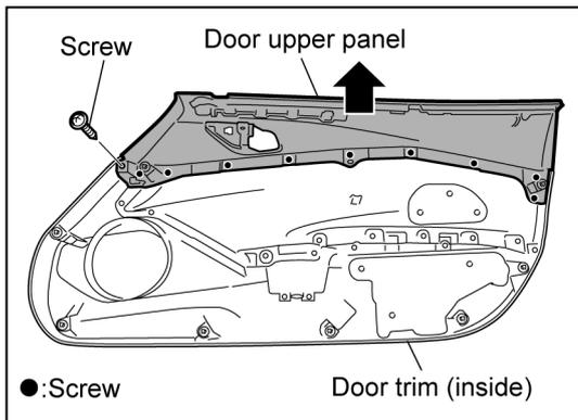
3. Remove the screws (10 places) on the inside of the removed door trim, and then remove the door upper panel (shaded part).
