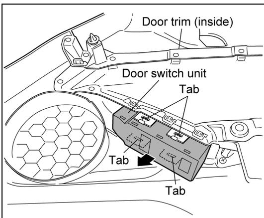
1. Turn the removed door trim inside, disengage the tabs (4 places) on the door switch unit, and then remove the door switch unit.
