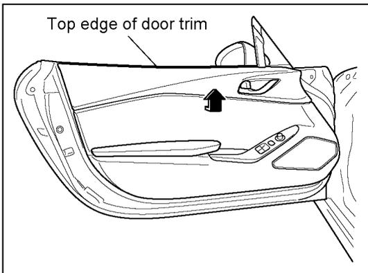
7. Lift up the door trim to disengage the catch at the top of the door trim.
