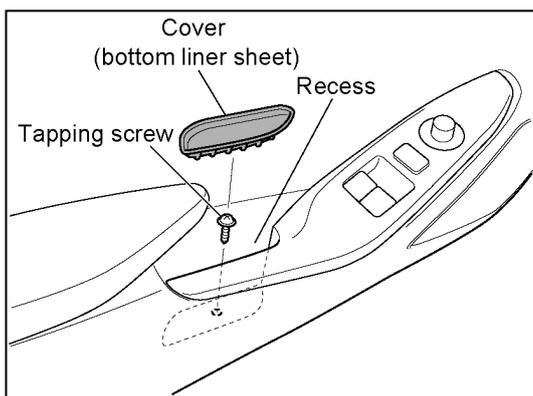
4. Remove the recess cover (bottom liner sheet).
