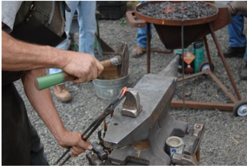
Forge welding a chain link
