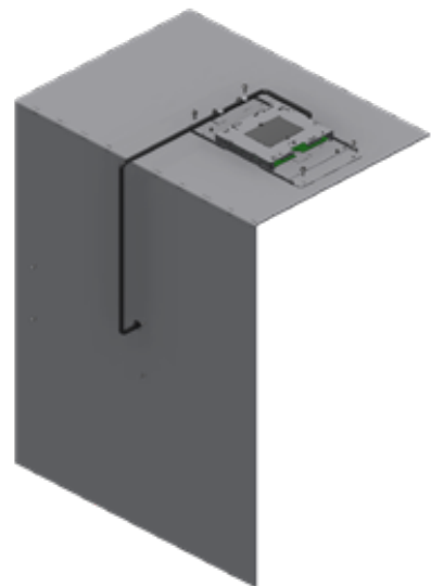
6.5' cable mounting – Display is mounted on fixture and processor is mounted top of car
