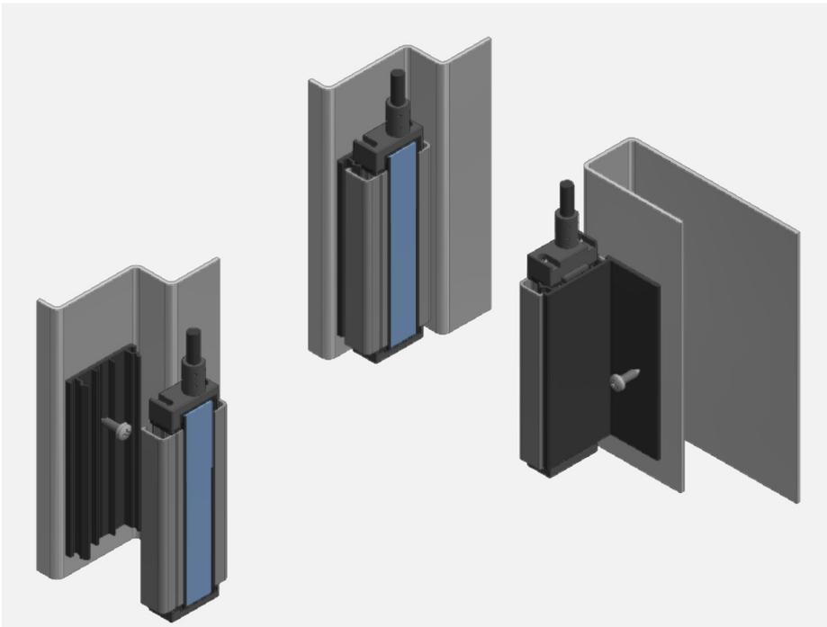
Fig 2: Strip Post Installation
