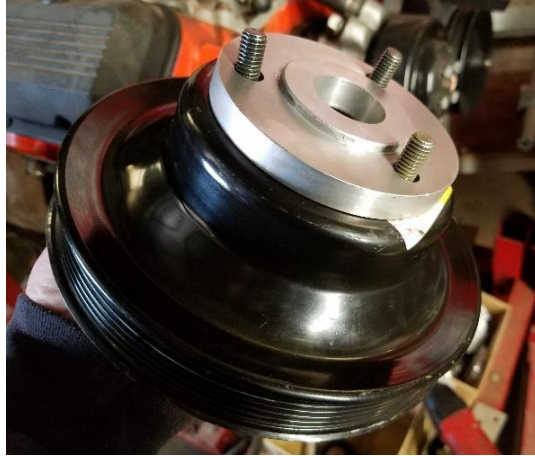
Above: SBC crank pulley and Kwik adapter. Note machined lip to properly center the pulley.
