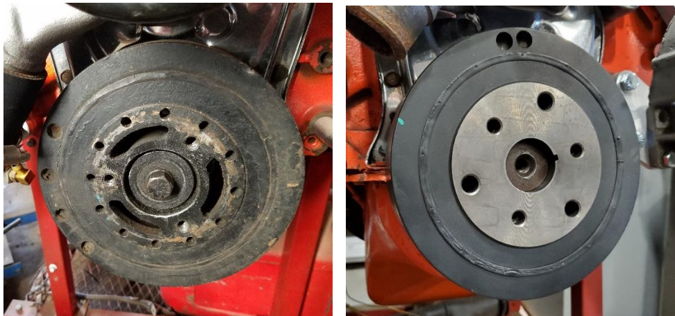
Above left: Mark IV balancer. Above right: Late Gen V and Gen VI balancer.
