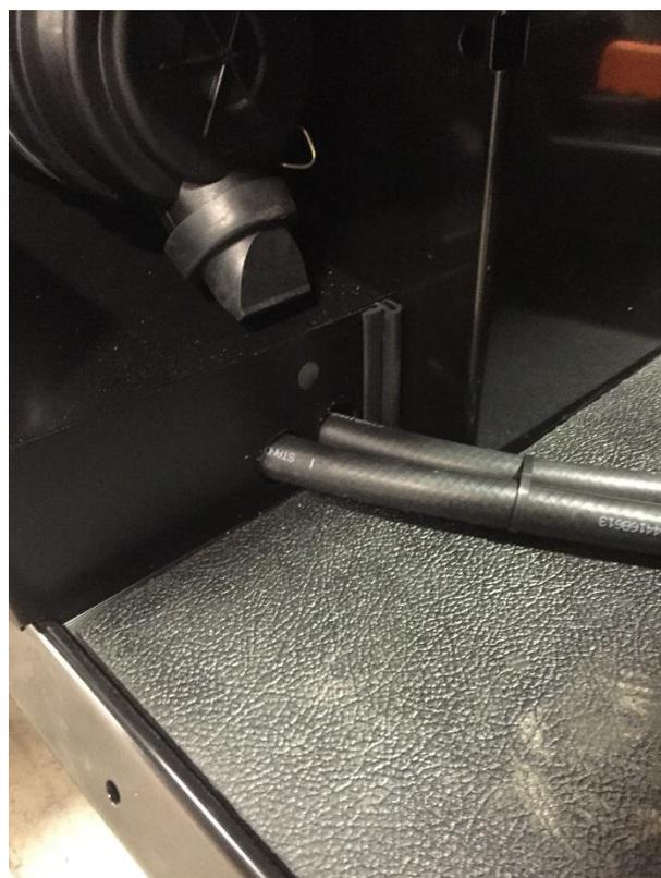
Run the hoses up and over the engine to the drivers side. There is a short hose that runs from each cylinder, you are going to eliminate that hose and attach the heater hose from the heater to where that hose was.
