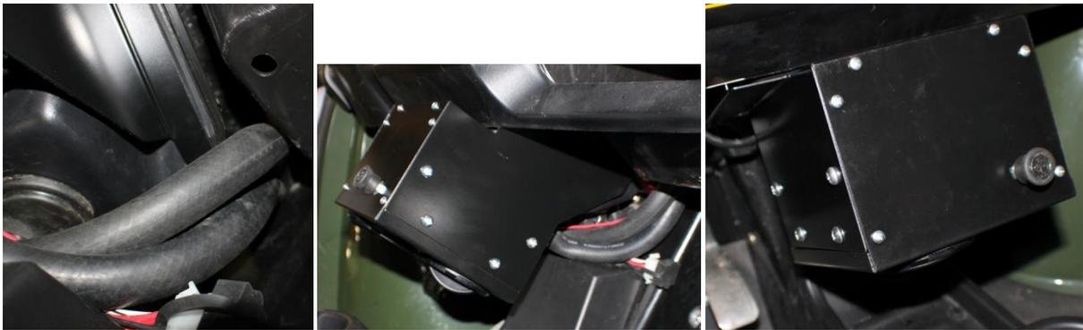
This is a self-grounded heater, meaning that once it is bolted in, that's what grounds it. There is only one wire needed to hook up to give the fan power. The power wire can be run back up where the heater hose was ran. There is an unused wiring harness under the hood and as seen in the picture we plugged the spade into the number "1" slot. You do not have to use this, but you need to wire it into a "keyed" power source, so that there is no power when the key is off.
