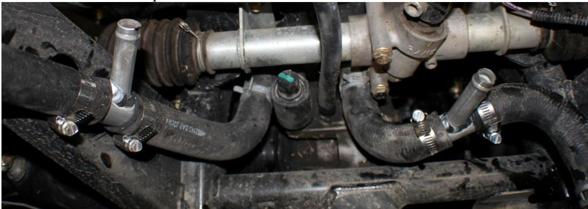
Now you can attach the heater hose to the splices. There is already a factory hole in the firewall that works for running the hose into the cab. Hose clamp the heater hose to the splice and run through the hole in the firewall. After the hose is run, you can reinstall the radiator. **Note: Do not fill with coolant yet.**
