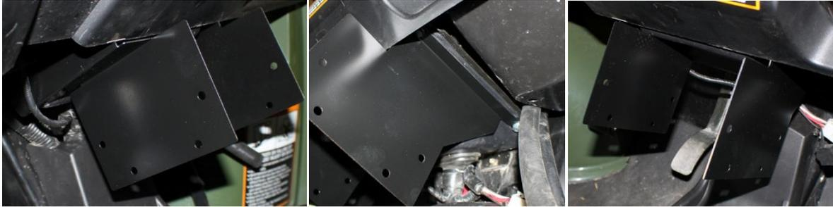
Now take the heater and attach the hose to the heater core fittings coming out of the back of the heater. It is easier to do this while the heater is not mounted to the brackets. After the hoses are connected take the heater and slide it between the brackets and line up the hose and mount it with the screws supplied.
