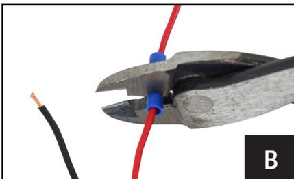
B. Crimp the supplied fuse holder onto the end of the RED wire and attach to the battery "+" terminal.
