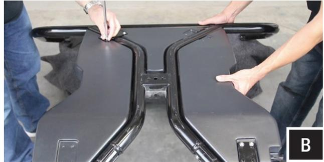
B. While holding the enclosure securely to the underside of the cage, loosely install the 5 brackets using the screws provided, attaching the front brackets first will help support the enclosure while attaching the other brackets
