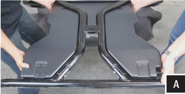
A. With one person on either side of the vehicle place the WP3-WC204A into location from the underside of the cage, place the back into position first, and then swing the front up into place.
