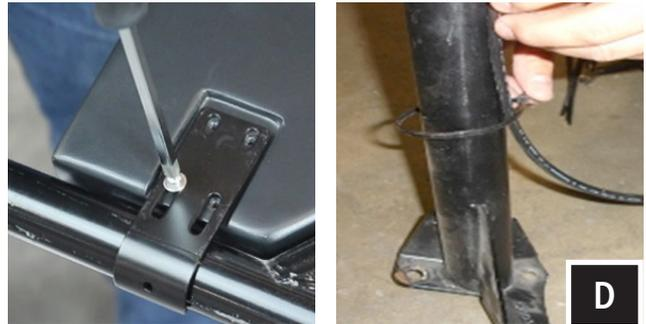
D. Using the zip ties provided, route the Power/Ground loom to the battery location away from any moving parts or sharp metal. NOTE: The 4 pin long cable is an audio output for adding an additional amplifier and speakers.
