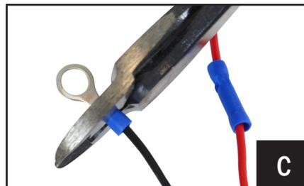
C. Crimp the supplied ring terminal to the BLACK wire and attach to the battery "-" terminal.
