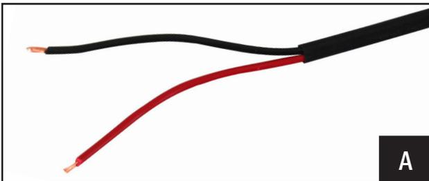
A. Cut the power/ground cable to length; be sure to leave enough wire at the battery location to wire to the battery, strip back approximately 4 inches of the black tubing to expose the red/black wires inside. Strip back 1/4"-1/2" of wire to make your connections.
