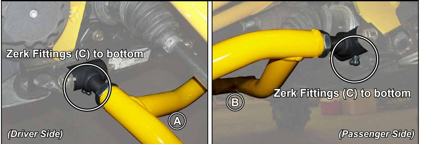
Fig. 2 - Install to Frame with stock hardware
