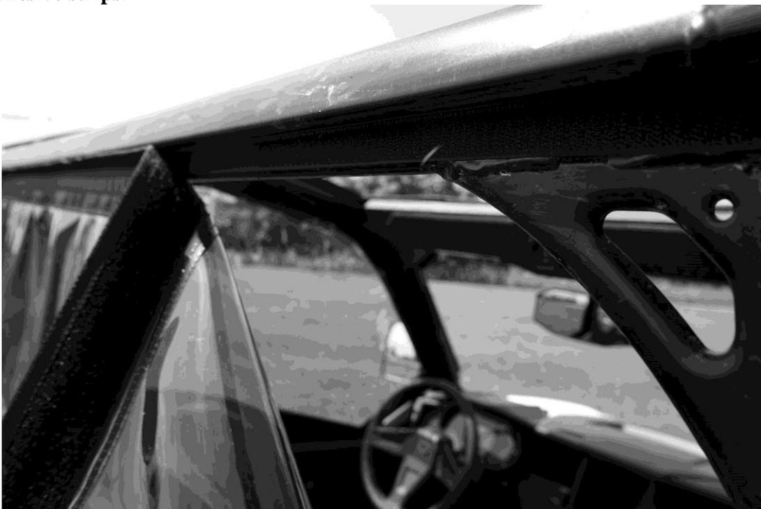
10. After the adhesive Velcro strips have been installed along the top and down the sides you can now place your rear window in the frame. Lastly mark where the bottom of the rear window sits on the vehicle and place the 48” adhesive strip flat on the vehicle so the bottom of the rear window pulls into the cab and attaches downwards.
