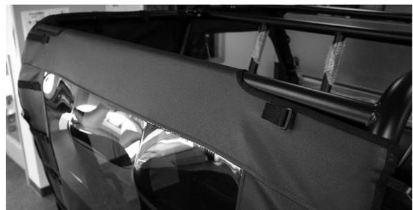
3. With the top and bottom of the Rear Window in place, now work your way down each side. You will see six strips of double-sided Velcro sewn perpendicular to the edge of the panel. At each of these locations you will wrap one of the 6" adhesive Velcro strips around the roll cage. Then wrap the double-sided Velcro around the adhesive Velcro as shown in the photos below.
