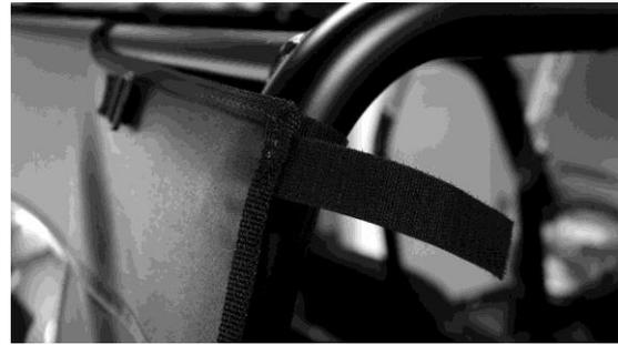
4. Now you are ready to install the door panels. As you will see, these have the same double-sided Velcro strips sewn perpendicular to the edges of the panel as the rear Window panel. With help from another, hang the door panel starting at the top. Make sure that the front and rear of the door panels are centered before marking and wrapping the roll cage with the 6" adhesive strips. It is best to start in the middle of the top and work your way to the front first. Then work your way to the rear.
