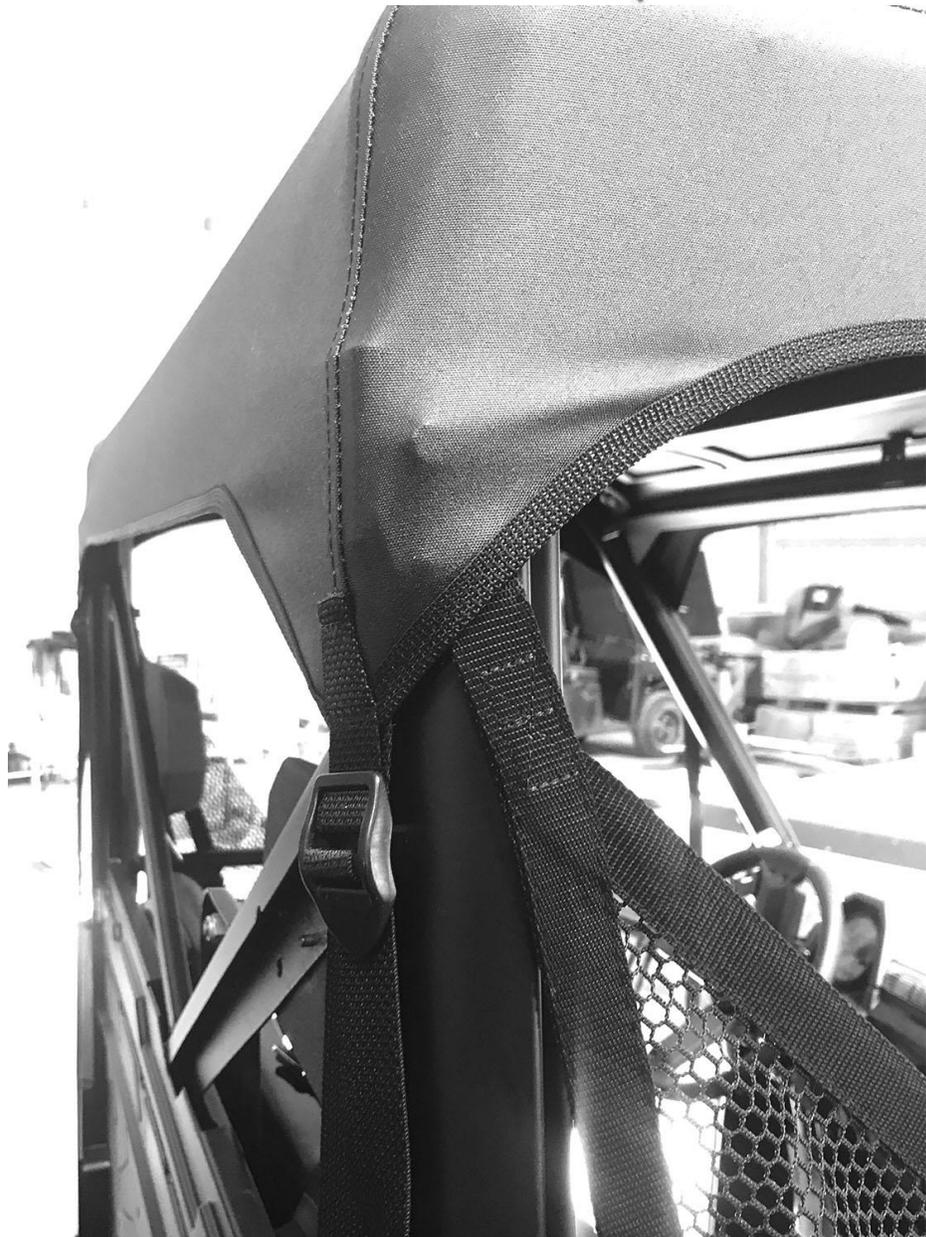
4. Moving to the front of the vehicle you will now need to raise the hood to reveal frame. Again take the looped end of one of the straps and run it around the frame just below the hood line. Then run the other end of the strap through the loop and pull it tight. Photo below shows how it should look.
