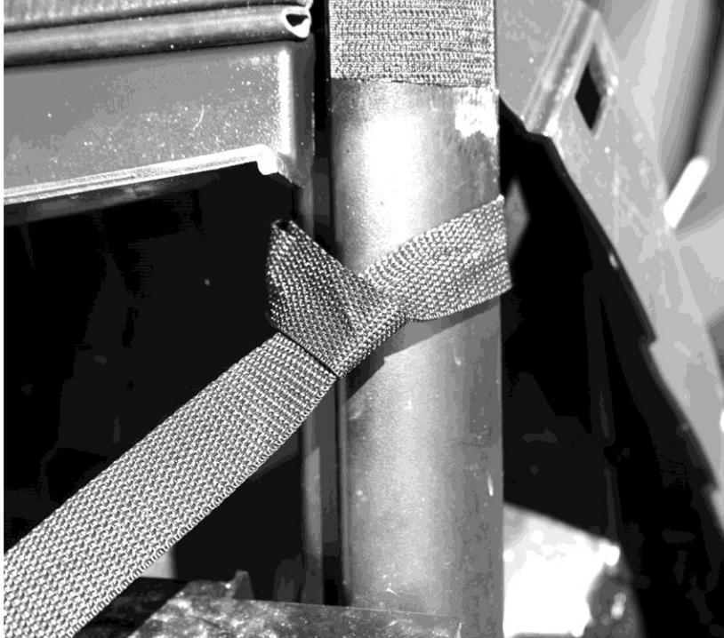
5. Now run the other end through the buckle in the front corner of the Top cap as you did in the rear and pull it tight. Now work your way around the top making sure that it is centered correctly and pulled as tight as possible.
