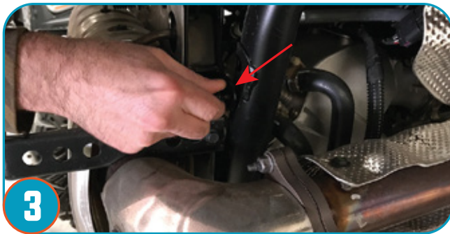
Remove the 2 M6 bolts holding the muffer support bracket to the chassis, on each side of the vehicle.
