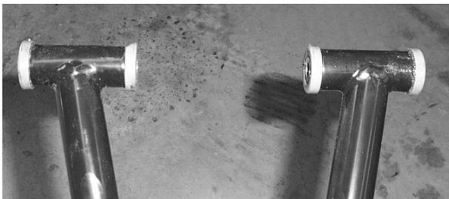
**NOTE: A press or a vise is suggested for removing and replacing the ball joints. Verify that the clip snaps into place after installing the ball joints into the new Control Arm**
