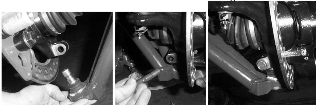
8. Place wheels back on RUV torque lugs to factory specifications.
