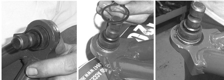
6. Use the factory nuts and bolts to connect the new Control Arms to the RUV frame. You will have left and right lower Control Arms.
