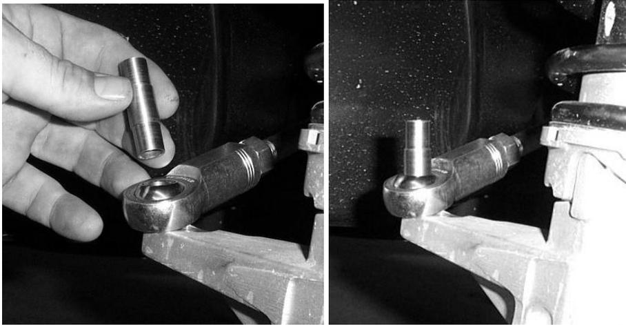
13. Place alignment cones onto the sleeve, on either side of the heim joint.
