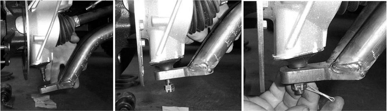
10. Remove the stock tie rod end and connect the new heim joint provided.
