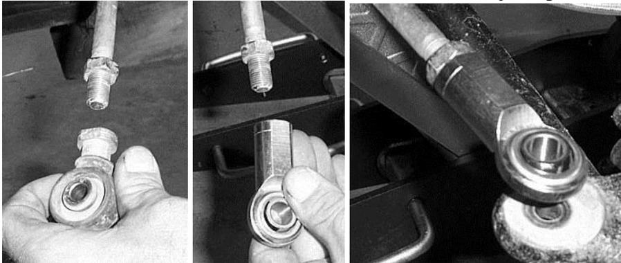
11. To connect the new heim joint to the knuckle assembly use the 10mm x 80m bolt, heim sleeve, alignment cones, 10mm washers, 10mm nut and 10mm lock nut.
