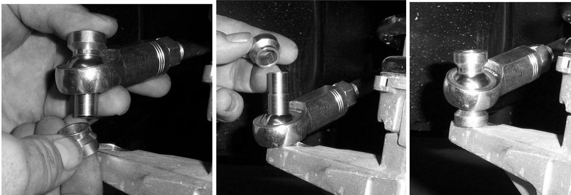
14. Place a 10mm washer onto the knuckle assembly and insert the 10mm x 80mm bolt through the heim joint, sleeve, and cones.
