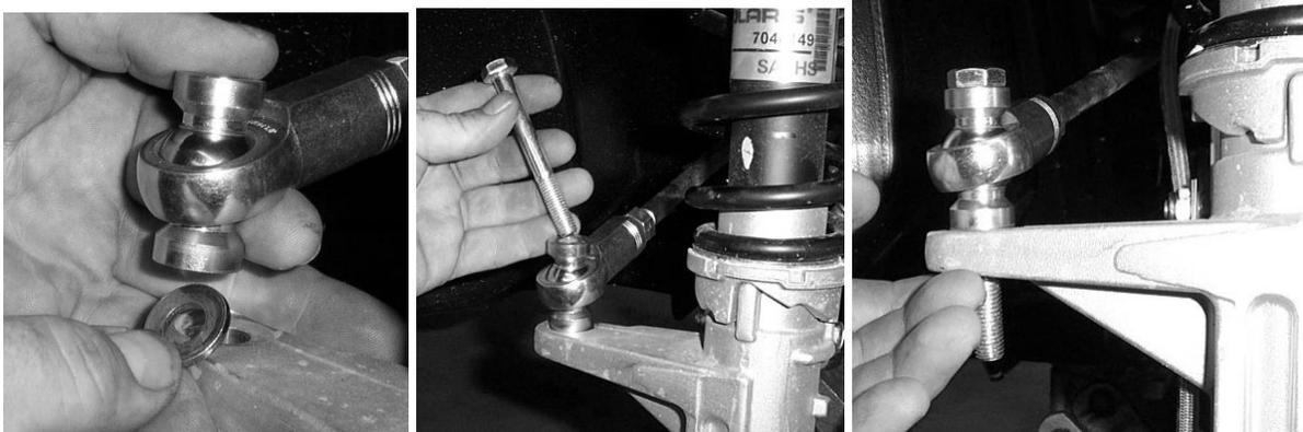
15. Place a second 10mm washer onto the bolt and secure it with the 10mm nut and then the 10mm lock nut.
