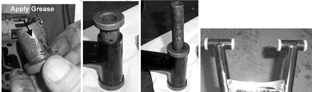
7. Install the grease fitting into the new arms before installation. **DO NOT OVER TORQUE THE FITTINGS.** Make sure to fill with factory approved grease.
