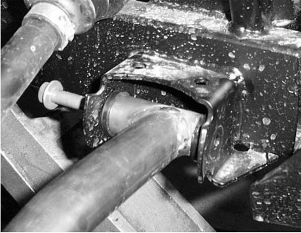
9. Reattach the hub assembly to the lower A-arm. Use the factory castle nut and cotter pin.
