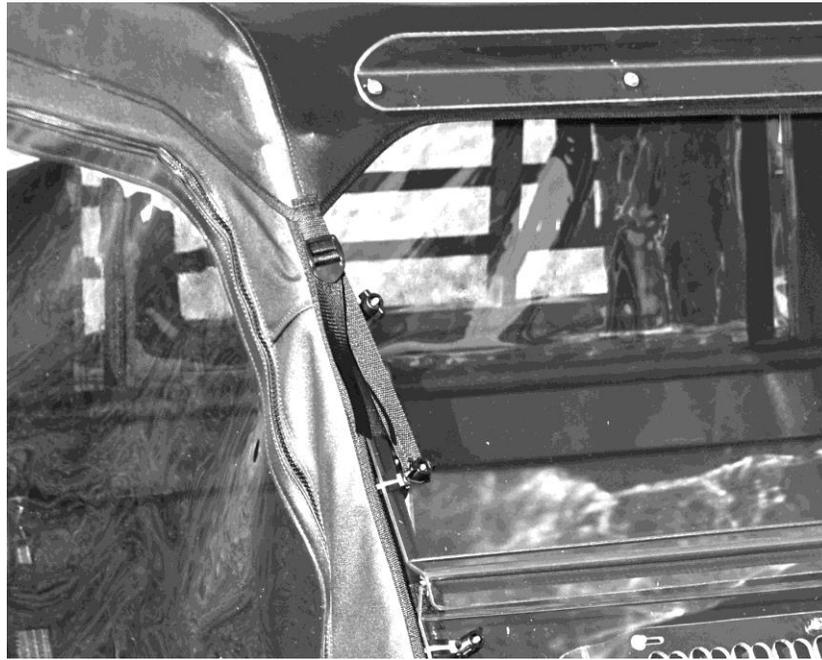
13. The rear of the Top Cap is held in place using the straps that have double-sided Velcro sewn in one end. Take the 6" adhesive Velcro strips and wrap them around the roll cage approximately 12" below the back of the Top Cap. Now take the end of the strap with the Velcro and wrap it around the bar and Velcro as tight as possible. Then take the other end of the strap and run it through the loop, pulling it tight. The photo below shows what it should look like.
