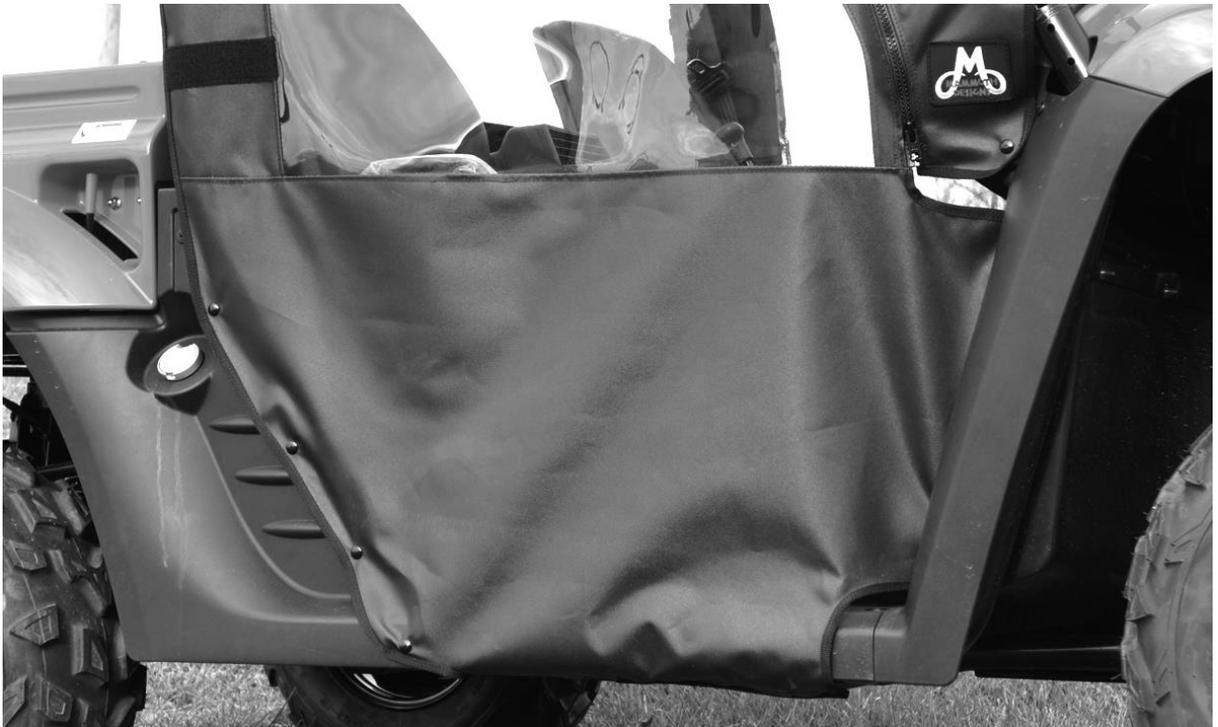
5. The front bottom section of the door has three snaps that attach inside the vehicle. They are reverse of the rear portion and will go on the inside wall of the foot well. See photos below.
