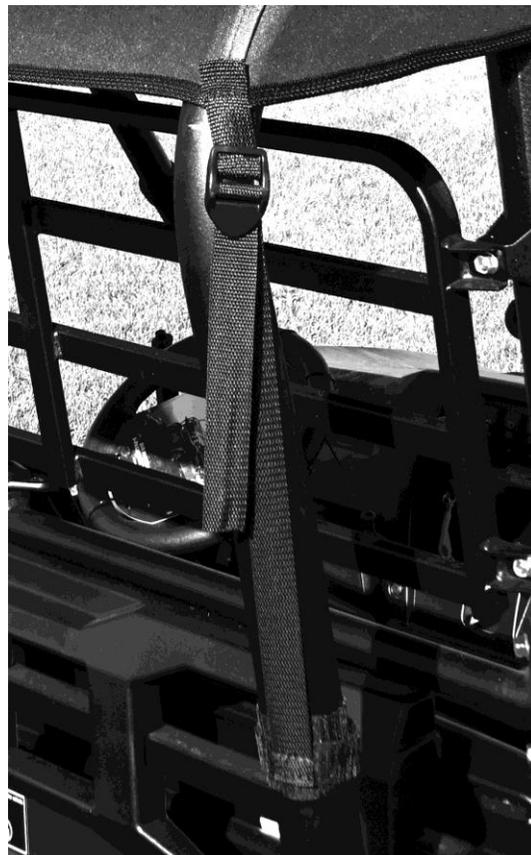
14. Once all the straps are in place run them through the buckles. Pull them tight making sure the top is centered and the side seams line up correctly along the roll cage. The diagram below shows how to lace the webbing through the buckle.
