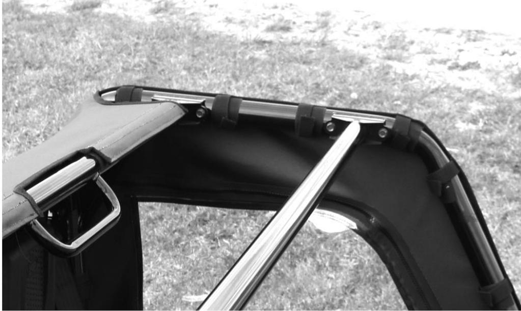
2. The rear edge of the doors has a 24" double-sided Velcro tab that will attach to the rear of the roll cage. Place the 24" adhesive strip on the roll cage to match up with tab.
