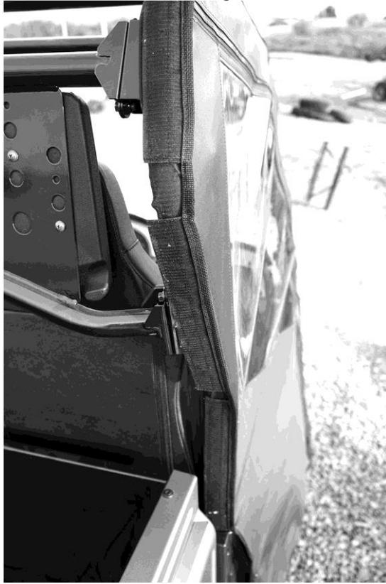
3. Once all the Velcro is in place the last thing to do is install the screw snap studs. **NOTE: The best way to install the snap studs is to put them in the sockets in the door first. Then push them into the plastic to make a mark. Then pull the screw stud out and screw it into the plastic where the mark was made. See Photos Below.**
