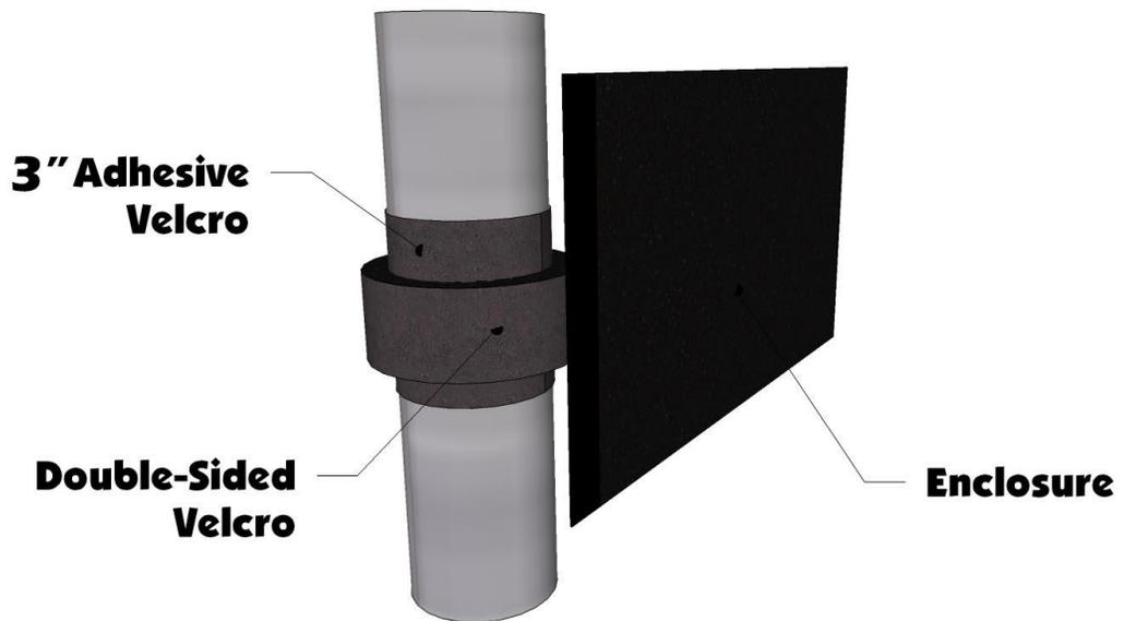
2. Next take the 38" adhesive Velcro strips and run it down the back of the roll cage facing towards the rear of the vehicle. Start at the bottom and work your way up the bar. You will see the double-sided Velcro tabs sewn along the back of the doors. See photo below.
