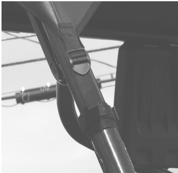
5. Then install the rear straps with the loop on the end. Run the strap around the end of the brace behind the seat and through the loop in the end of the strap. See Photo Below
