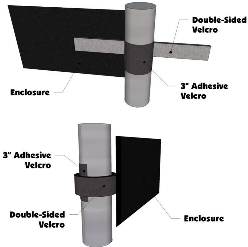
6. The top of the rear window will attach to the bar as shown below:
