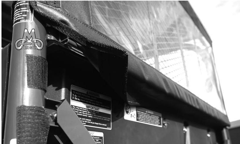
5. Now pull the rear window up and attach it to the top bar across the back of the roll cage. The top and sides of the rear window has double-sided Velcro sewn along the edges. At
