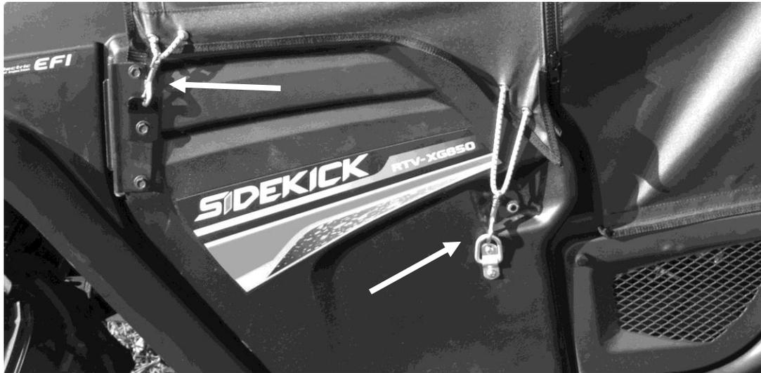
9. Check proper fitment around the perimeter of the door, and make any adjustments necessary. The door should have some slack to allow for proper function of the zipper. If the material is pulled too tight the zipper will catch leading to difficulty when opening or closing the door.
