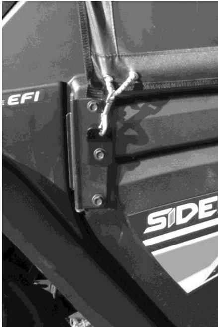
6. Hold the plate from the D-ring bracket on the door approximately 1in from the bottom of the recessed latch and 3in from the edge of the door and mark the position of both holes. This position is important because if the plate is too close to the edge of the door the mounting bolts will hit the door jam and the door will not close properly. Make sure the door is open and use a  $\frac{1}{4}$  drill bit to drill the mounting holes for the plate.
