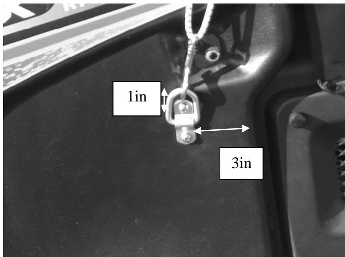
7. Attach the D-ring and mounting plate using the provided  $\frac{1}{4}$ -20 x 1.75in bolts, fender washers and lock nuts. Tighten completely.
