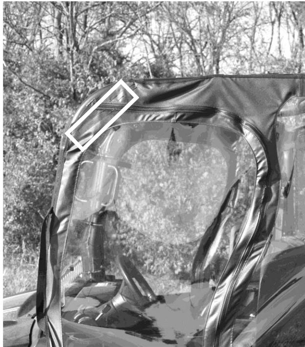
4. Attach the 3 pieces (2in, 4in, and 12in) of 1in adhesive Velcro to the UTV following the profile of the UTV and the bottom edge of the door.
