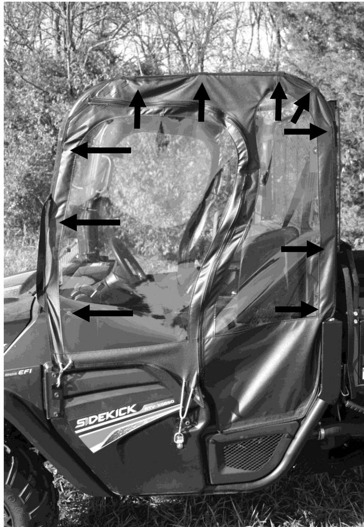
3. Place the 2in x 7in adhesive backed Velcro strip in the top, front corner of the roll cage. Align the edge of the Velcro with the edge of the steel reinforcing plate.
