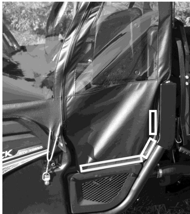
5. Remove the center door hinge bolt and mount the metal hinge bracket. Be sure to tighten bolt completely.
