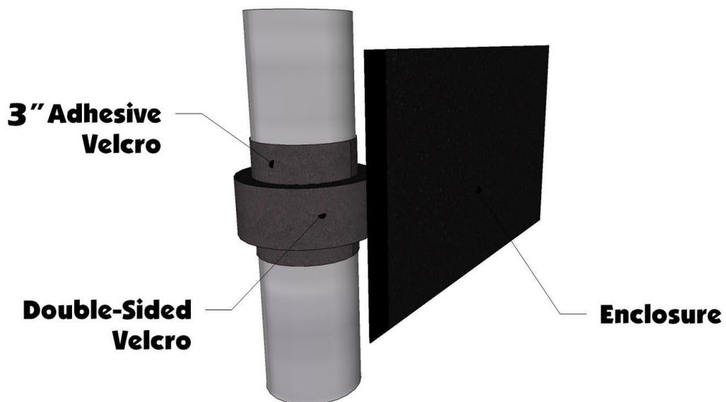
2. The following image shows the approximate location of each of the 10, 3in Velcro strips that need to be placed on the roll cage. Extras are provided in case some are placed incorrectly during the initial placement.
