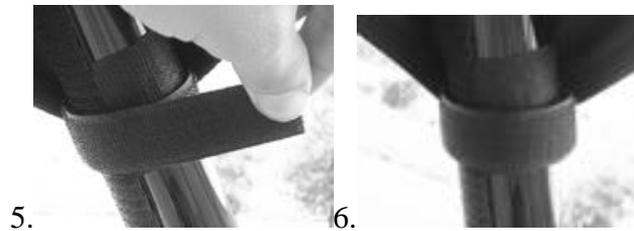
5. Clean the surface of the roll cage tube. Note the position of the Velcro strips down along the sides of the front window and install three 8” adhesive Velcro strips lengthwise down the left front of the roll cage, on the outboard sides of the steel tube. Attach the left side of the enclosure. Repeat these steps for the right side, but pull the window tightly toward the right to minimize waviness or wrinkles in the front window then attach.
