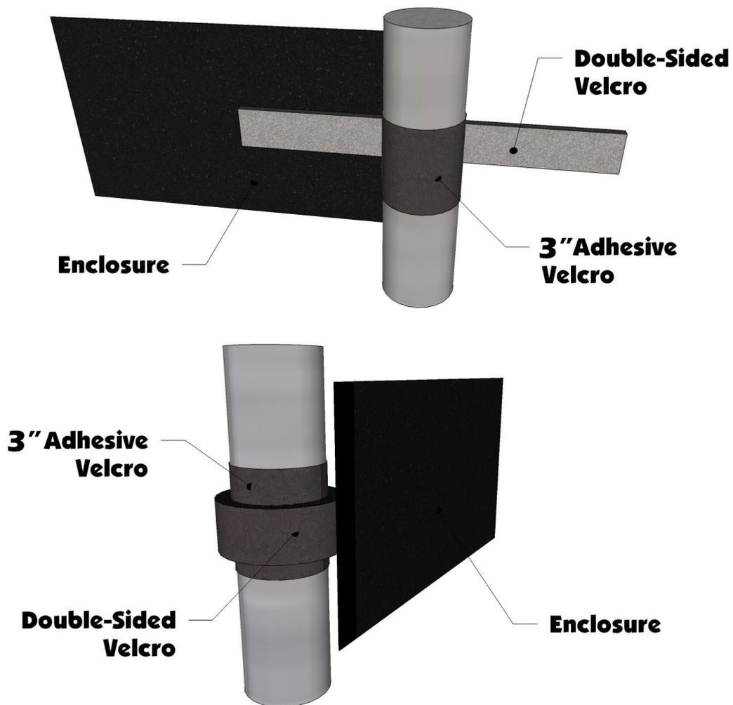
6. Now work your way down the back of the door attaching the adhesive Velcro strips that match up with the Tabs sewn along the edge.
