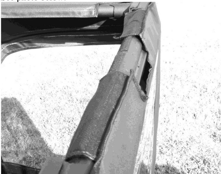
5. Then place the rest of the 10" adhesive strips down the sides of the rear window to match up with two tabs sewn along the edges. See photo below
