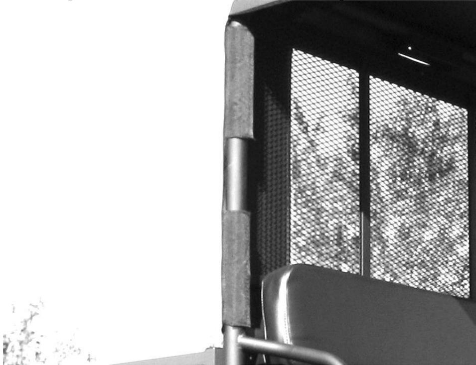
6. In the top corners, place a 3" adhesive strip on the inside of the bar where the double-sided Velcro strips are sewn perpendicular to the edges of the rear window. Photos below shows how this works.
