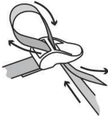
14. Now move to the rear of the vehicle and install the straps with Velcro to the roll cage between the door panel and the rear window panel. Run the strap out between the two panels as shown in the photo below. Be sure to use the 6" adhesive Velcro strip and wrap it completely around the bar for maximum holding strength.
