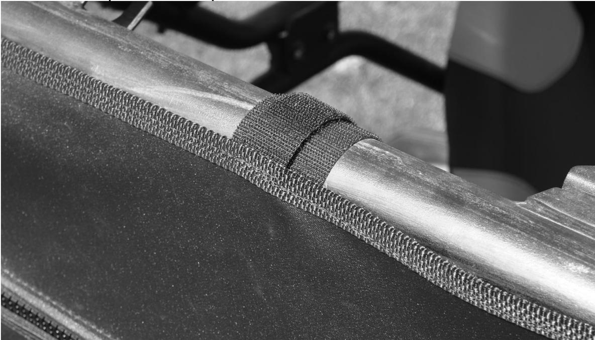
7. Next step to install the side door panels is to install the snaps along the bottom of the door panels to the plastic doors on the Teryx 4. As you will see there are four snaps that attach to the outside of the vehicle and six snaps that attach to the inside of the plastic doors.
