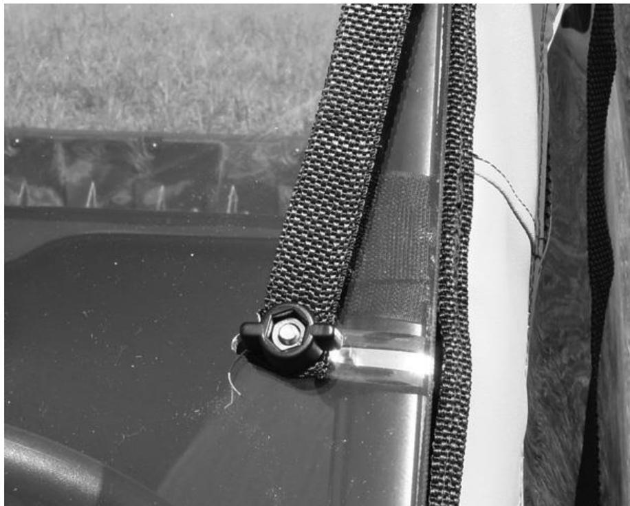
13. Next run the strap up and through the ladder lock buckle as shown in the photo below.
