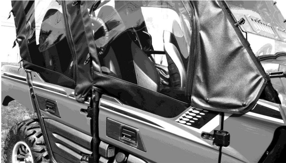
8. To install the rear window panel you should begin by installing the three double-sided Velcro strips down both sides which will go under the door panels along the back edges. Make sure to line up the grommet holes along each edge so that they are close to being side by side.
