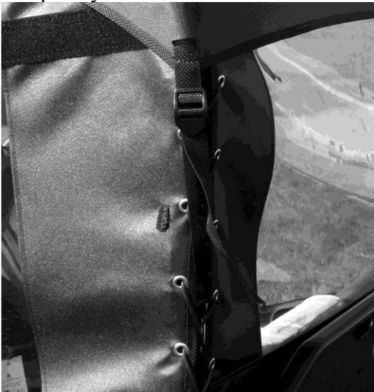
15. Run the strap up and through the ladder lack buckle as you did with the front and pull tight. Now you must make sure that the top is properly centered and pulled tight over the top. Make sure that the top is lined up so that the snap down the middle will snap to the door panel.
